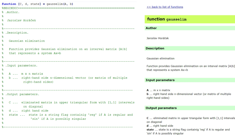
Figure 12.3: Example of OcDoc text documentation structure within an .m file (left) and the resulting .html page (right).
