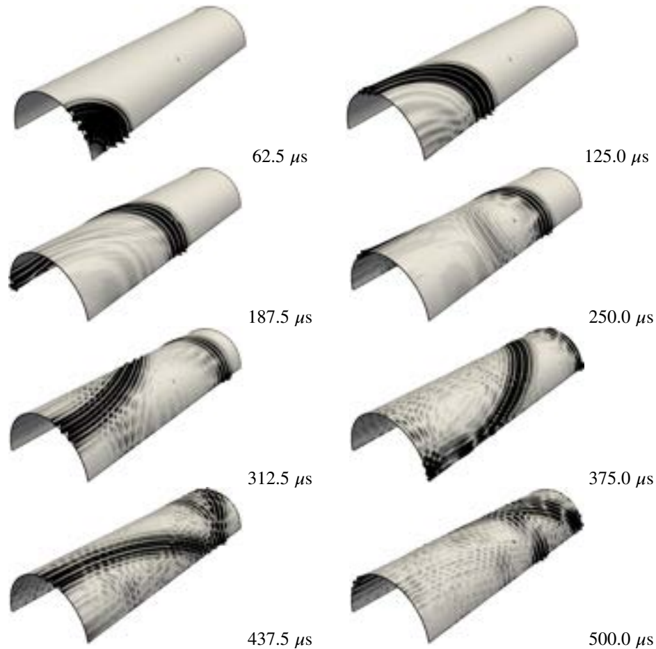
FIGURE 13 Half-pipe shell with an open crack. Snapshots of the propagating waves at 62.5 \mu\text{s} intervals, from 62.5 \mu\text{s} to 500.0 \mu\text{s} .
